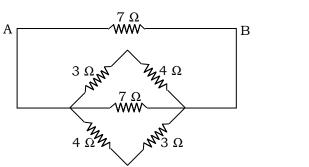
Calculate the equivalent resistance between the points A and B in the given Figure.
